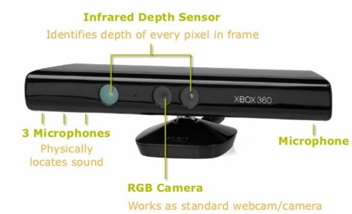
Hinh 3: The structure of the MS Kinect v1 sensor.
