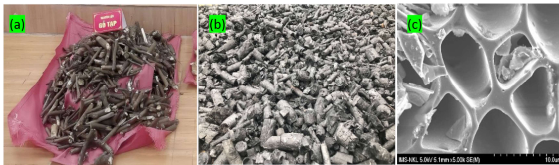
Figure 5. Experimental Images of Biochar Production and Analysis: (a) Raw wood materials, (b) Biochar derived from wood materials, (c) SEM image of the biochar
