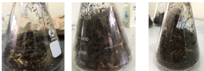
Figure 2. Visualization of hemp hurd weight reduction after 30 days of cellulose-degrading microbial treatment
